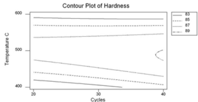
**Fig. 6: The contour plot of the hardness (HRB) as a response and cycling temperature and No. of cycles**
